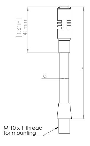
Length (L) 100mm (3.9") Model No. C 31 C 32 + C 32/SR C 33 + C 33/SR C 34 + C 34/SR C 35 + C 35/SR C 36 + C 36/SR 200mm (7.9") 300mm (11.8") 400mm (15.75")
