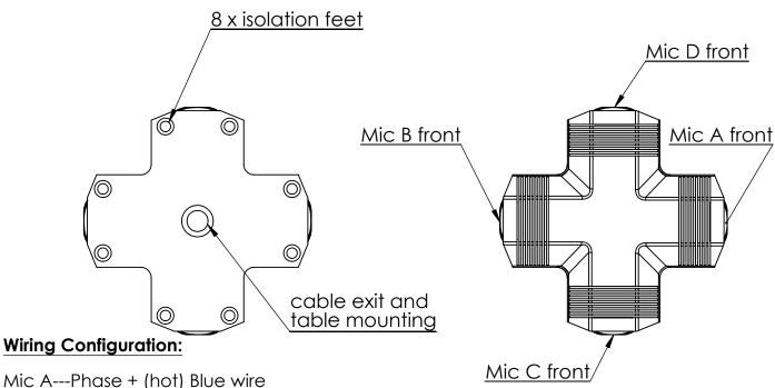
Mic A---Phase + (hot) Blue wire Phase - (cold) White wire ground---screen
