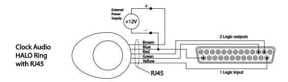
Figure 4. Example of wiring of a *Litetouch Halo ring and touch pad* to a SoundStructure device connected to logic output 1 (physical pin 2) and logic output 2 (physical pin 3) and logic input 1 (physical pin 14). Each *Litetouch Halo ring and touch pad* requires 2 logic outputs and one logic input pin from the SoundStructure device
