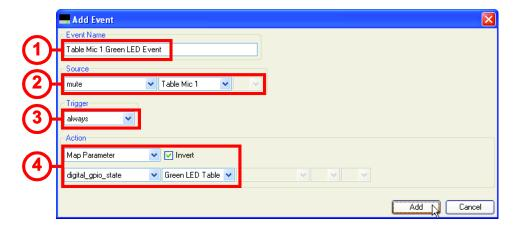
Figure 11. Defining the green LED event for Table Mic 1 based on the mute state of the microphone. Note the invert option is selected so that the green LED only lights up when the microphones are not muted
