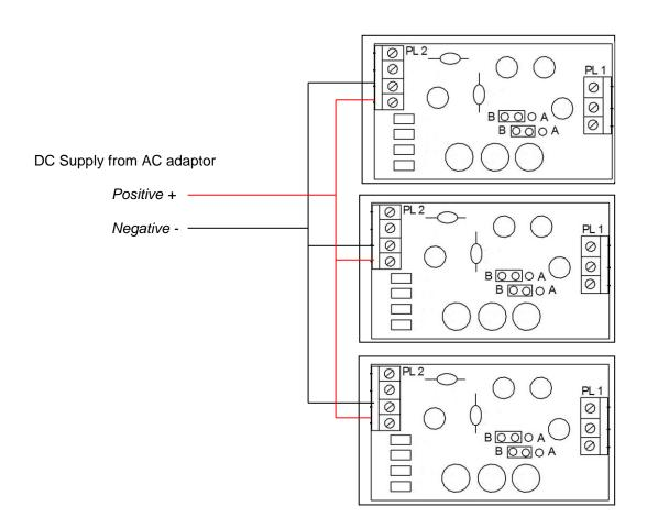
The Current taken by each CAP002 is very small approx 5mA. An AC power adaptor with 100mA capability will be able to power up to 20 CAP002 circuits.
