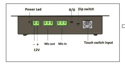
Mic In: pin 1 gnd, pin 2 phase + pin 3 phase - Mic Out: pin 1 gnd, pin 2 phase + pin 3 phase - R/G red / green mic live designation switch using TS001 / CH32.
